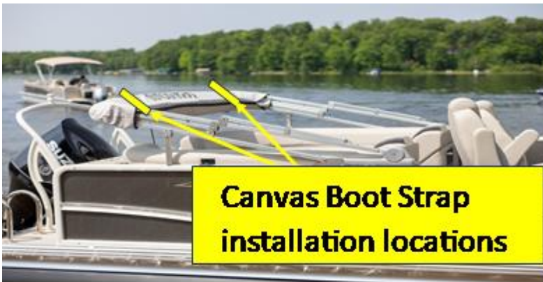
Canvas Boot Strap installation location (secures frame/boot for high-speed travel)
