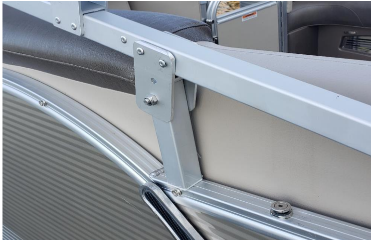
Rear support foot mounted on autobimini lite aluminum 4 th riser and positioned to avoid interference with boat upholstery.
