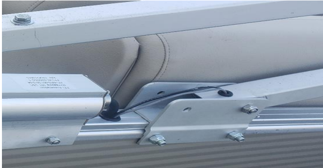
Navigation wires routed in rear riser, rear arch bracket and actuator grommet
