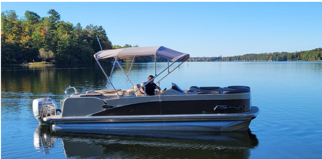
autobimini lite installation with front support arms installed
