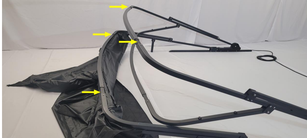
Arches – connector tube - riser arm assembly shown bolted together (make sure all the connector tubes are same width for a square frame assembly)
