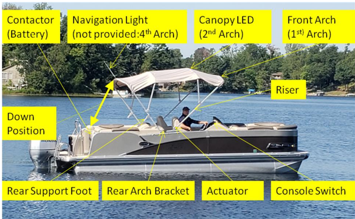
autobimini lite installation (shown without front support arms installed)
