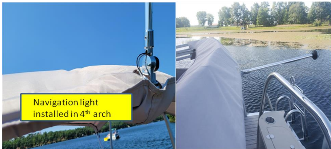
autobimini lite with navigation light installed in 4 th arch
