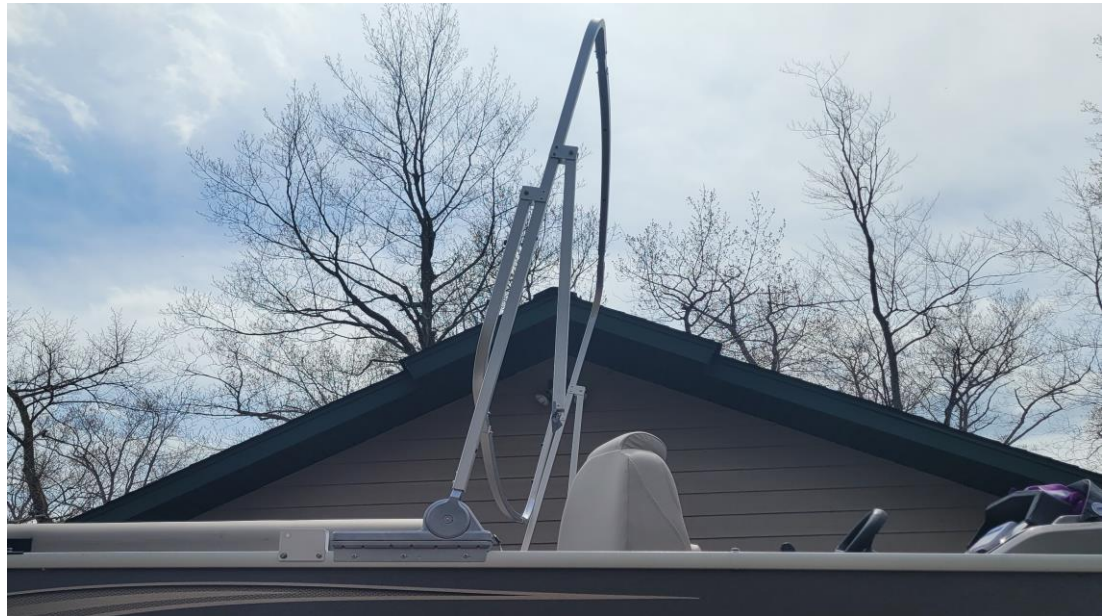
autobimini actuator installed, shown with wire routed through playpen (hidden)
