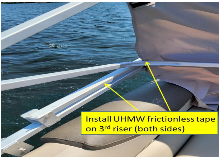
UHMW (ultra high molecular weight) film allows frictionless sliding
