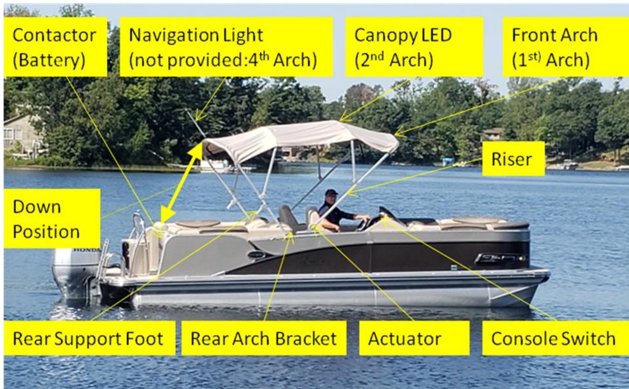
Installation with component names and relative locations
